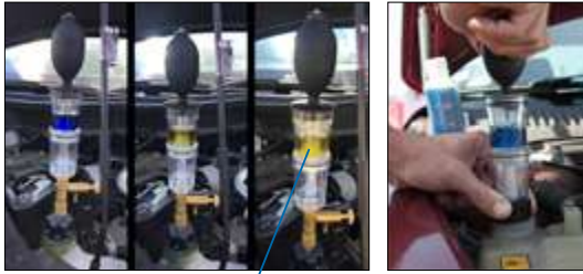
Yellow liquid = cylinder head gasket out of order
